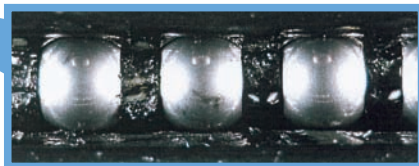
Detail view of the ball cage
