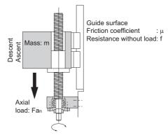
$Fa_6$ : Axial load during downward deceleration (N) m: Transferred mass (kg)
