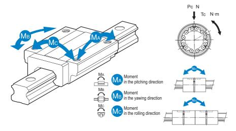
$\begin{array}{lll} P_c & : Radial \ load & M_{\text{A1}} & : \ Moment \ in \ the \ pitching \ direction \\ T_c & : \ Moment \ in \ the \ torque \ direction & M_{\text{A2}} & : \ Moment \ in \ the \ pitching \ direction \end{array}$
