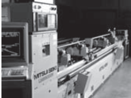
Automatic lead-measuring machine using a laser
