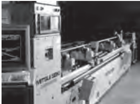
Automatic lead-measuring machine using laser
