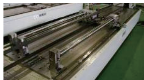
Appearance of the test machine (high-speed durability test)
